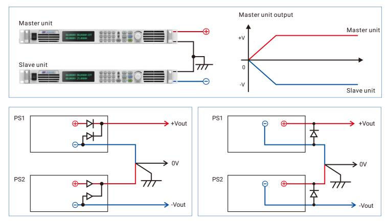
The power supply below 200A has been connected with anti reverse diode, so the external diode isn't needed in the actual connection, and the 200A power supply needs to connect the diode.
