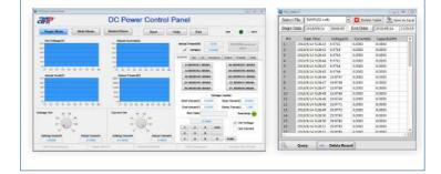
When the communication port has more than one power supply connection, it enters the Multi Mode interface. Supports switching control or display current power supply's settings.
