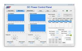
When the communication port connects the power supply that is the Master unit, it enters Master/Slave interface. The Master/Slave interface only maintains communication with the Master unit, and the parameters are synchronously written to the slaves.
